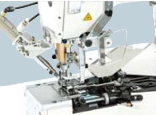
Pneumatic top and bottom thread trimming device
