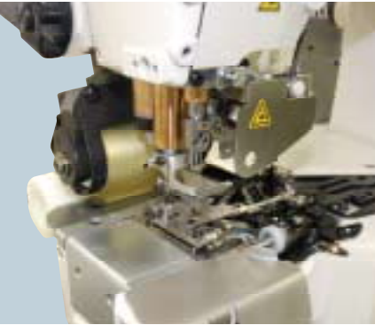
Pneumatic type bottom thread trimming device
