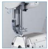
. The maximum alternating vertical movement is 6.5mm.
