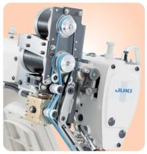
New type belt feed mechanism
