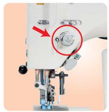
Active tension mechanism
