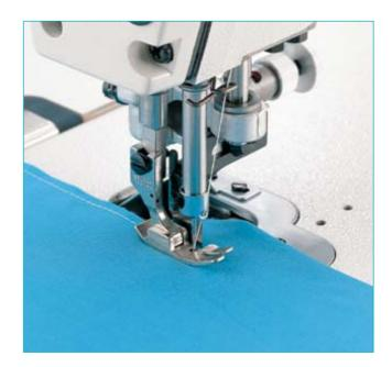
The maximum stitch length for the DLM-5200N has been increased to 5mm.
