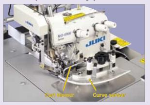
Automatic shirring is also possible at desired sections of the material by programming sewing data. The machine adopts an air-driven feed mechanism for feeding materials while preventing the material from slipping off the needle entry point.
