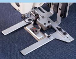
Sewing labels (FU05 type inverting clamp device)
